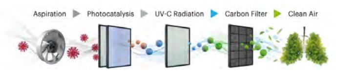
Using extractors, the air in the room is introduced into the AIRISYS disinfection and purification system. A pre-filter retains larger elements such as hair, insects, etc.
